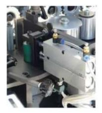
**Cutting Shears Unit**Powerful cutting shears up to 3 mm edging thickness
